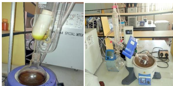
Figure 1: Soxhlet Extraction and Purification of Neem Seed Oil
