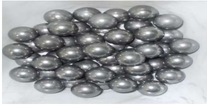
Figure 2.0: Tungsten carbide milling balls of 10 mm diameter with the average weight of 7g delete noimportant
