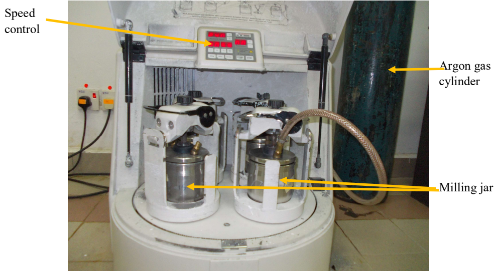
Figure 3.0: Ball milling operation set up using argon gas
