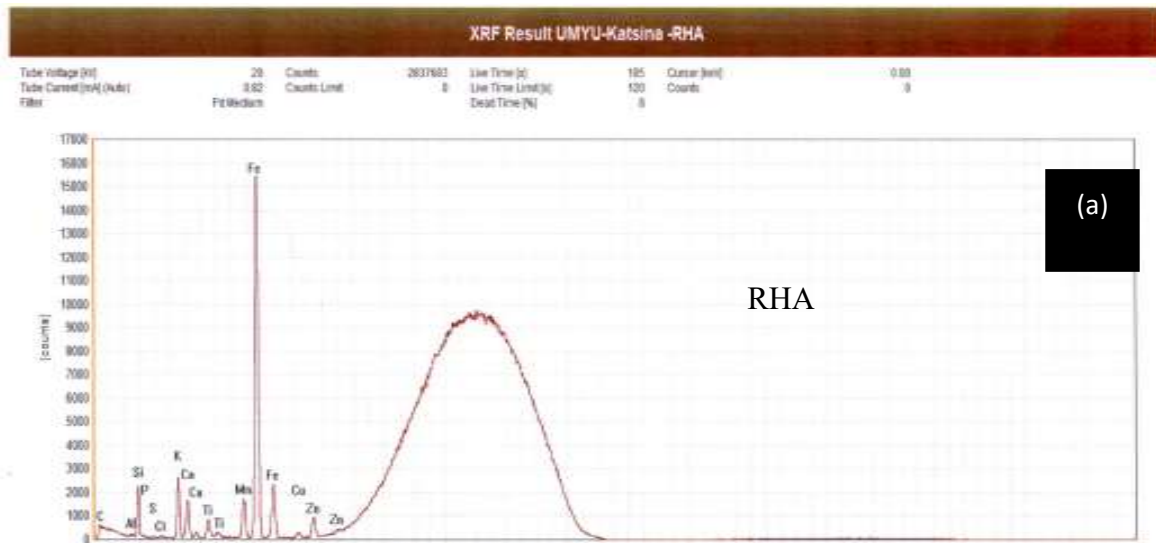
Fig. 7: A graph of XRF spectra showing a (a) the peaks and background at a particular % concentration and (b) plot of peak values of uncommon elements
