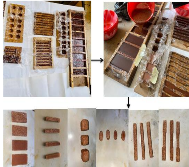
Figure 2: Sample production of the Composites Reinforced with Doum Palm Kernel Powder
