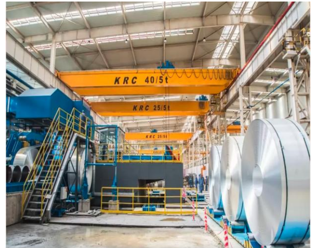
Figure 2: Double-girder crane system (Source: https://krccranes.com/wpcontent/uploads/Aluminum-Plant-KRC-Double-Girder-Crane.jpg.webp )
