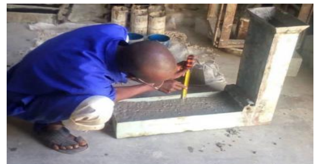
Plate V: PA test (L-box)
