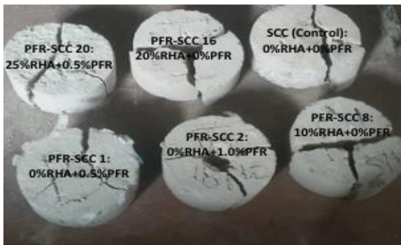
Plate XI: SCC/PFR-SCC Specimens (After Impact Blows Showing Different Failure Modes)
