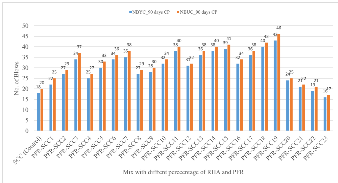
Figure 5: Impact blows responsible for yield (first) crack and ultimate crack for PFRSCC mixes (90 days curing period)
