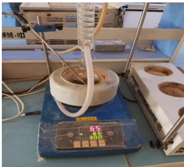
Figure 2: Experimental Set-up for the Mahogany Seed Oil Transesterification
